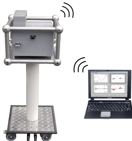
Figure 9: The ICMflex for simultaneous measurement of PD and TD
