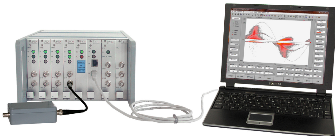
Figure 1: The ICMsystem was the first instrument to provide a coloured phase-resolved pattern.
