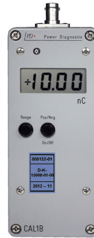
Figure 7: CAL1B calibrator with 100 pC up to 10 nC.
